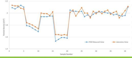
RESULTS SHOWN TO THE LEFT ARE ACTUAL PLANT TRIALS CONDUCTED BY CHPP STAFF AND ANALYSED BY 3 SEPARATE LABORATORIES. ALTHOUGH THERE IS OFTEN A SMALL DIFFERENCE BETWEEN THE MEASURED AND LABORATORY VALUE, THE PDM ALWAYS TRACKS CHANGES WELL, SHOWING THE GENERAL TREND AND ANY ALTERATION IN STREAM QUALITY. FLOTATION TAILINGS WAS BEING MONITORED.
